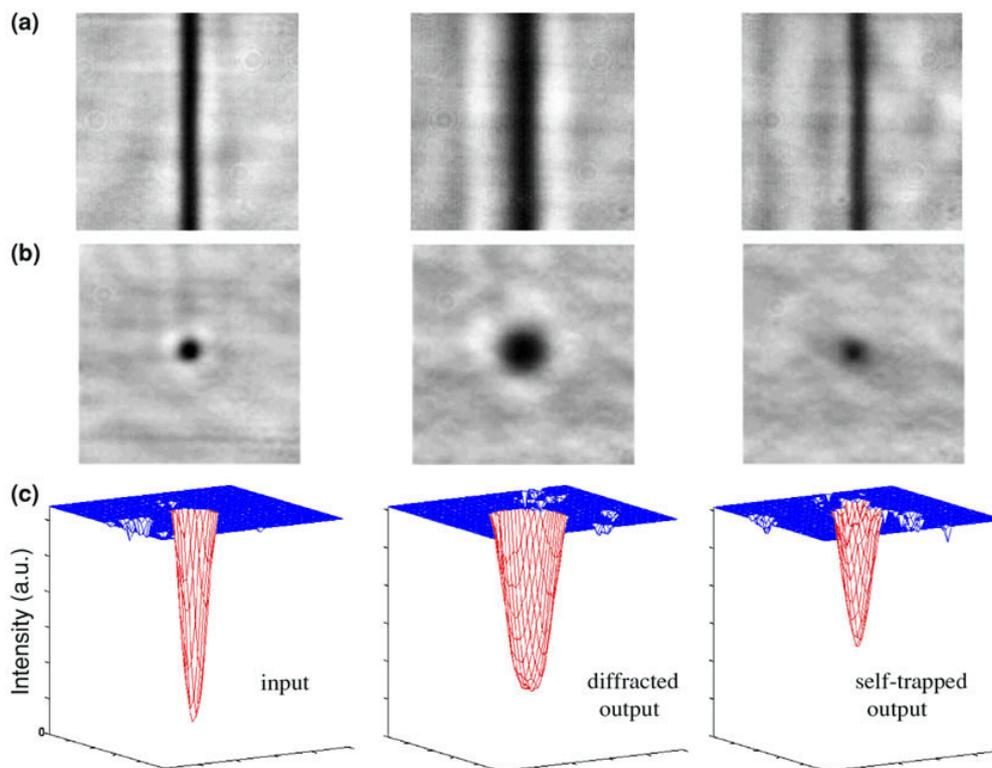
**Figure 4.** The self-trapping of a dark partially coherent beam. Shown are photographs of the transverse intensity patterns from (a) a dark stripe beam and (b) and (c) from a dark vortex beam taken at the crystal input face (left), the output face with linear diffraction (middle), and the output face with nonlinearity (right).
