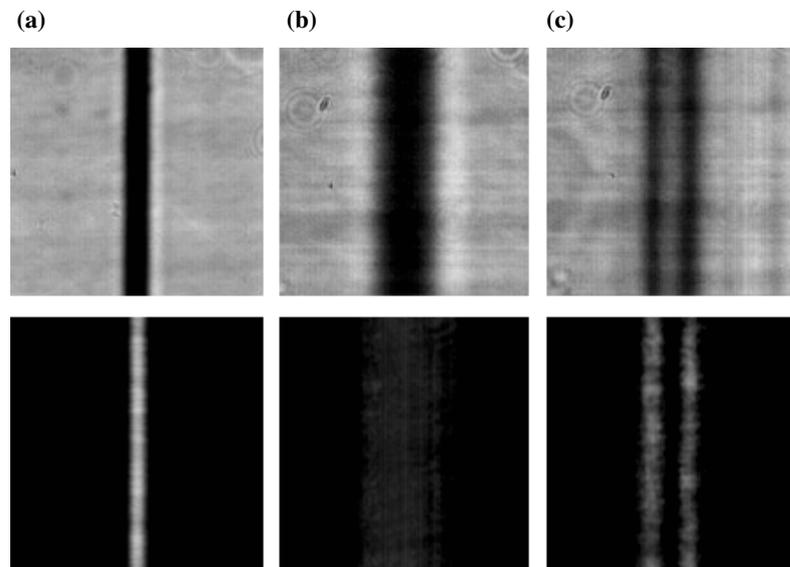
**Figure 5.** Photographs showing the self-trapping of a Y-splitting incoherent soliton (top) and the guidance of a probe beam (bottom) by the soliton-induced Y-splitting waveguide: (a) input, (b) output with linear diffraction, and (c) output with nonlinearity.
