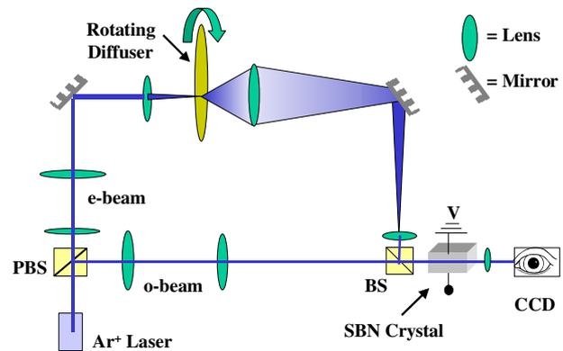
**Figure 1.** A typical experimental set-up for incoherent solitons. An argon ion laser beam is split into the o-beam and e-beam by a polarizing beam-splitter. The e-beam is sent through a rotating diffuser before recombining with the o-beam at the input face of an SBN crystal. Amplitude and phase masks (not shown) are used, as needed.
