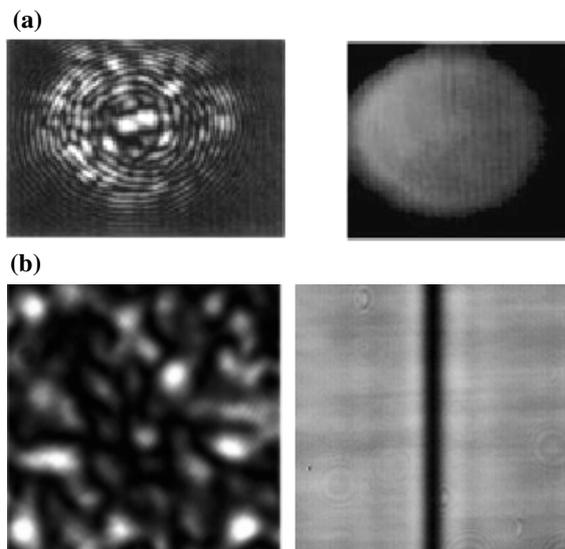
**Figure 2.** Photographs showing the non-instantaneous response of the photorefractive crystal: (a) interference patterns of a speckled beam and a uniform background beam; (b) intensity patterns of a speckled beam bearing a dark notch (left, diffuser stationary; right, diffuser rotating).
