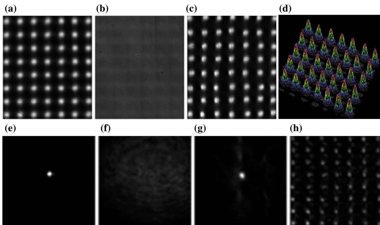
**Figure 7.** Spatial soliton pixels of partially incoherent light. Shown are intensity patterns from (a) the input, (b) output with linear diffraction, (c) output with nonlinearity, and (d) output 3D-intensity plot of (c). The bottom row shows a Gaussian-like probe beam at (e) the input, (f) linear output, (g) output with soliton-induced waveguides, along with (h) a plane-wave probe beam guided into waveguide arrays.
