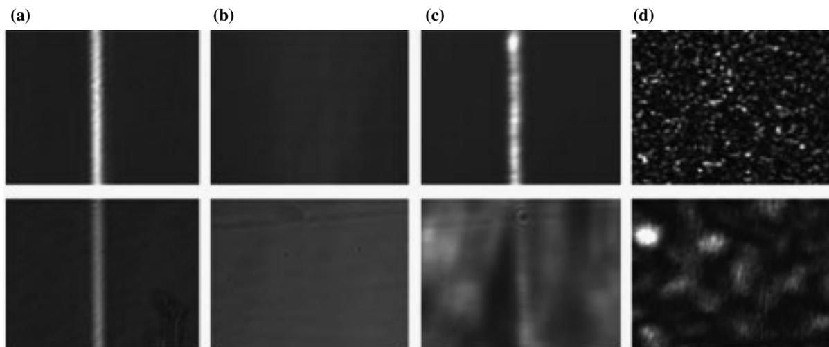
**Figure 6.** Experimental observation of a stable (top) and unstable (bottom) anti-dark soliton on a partially coherent background beam. Shown are photographs of (a) input beam, (b) output diffracted beam, (c) output self-trapped beam, and (d) speckled background beam.
