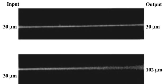
**Figure 3.** Self-trapping of a bright partially coherent beam. Shown are top-view photographs of the self-trapped (top) and normally diffracting (bottom) bright beams propagating inside the crystal.
