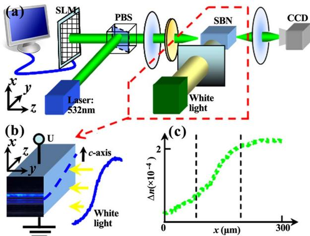
Fig. 2. (Color online) (a), (b) Schematic of the experimental setup. A biased SBN crystal is illuminated by nonuniform white light from  $x$ - $z$  plane, while the Airy beam is launched along the  $z$  direction. (c) Plot of induced refractive-index change along the  $x$  direction where two vertical dashed lines define the graded index area for beam control.
