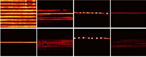
Fig. 4. (Color online) Experimental results. Upper row, first column, 1D lattice; lower row, first column, initial probe beam; upper row, results with lattice; lower row, results without lattice; second column, linear diffraction; third column, output with focusing nonlinearity; fourth column, output with defocusing nonlinearity. The bias field and crystalline  $c$  axis are along the vertical direction.
