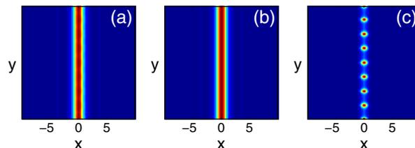
Fig. 3. (Color online) (a) Initial intensity pattern of the stripe soliton in Fig. 1(c) under 2% perturbations, (b) output intensity of the perturbed soliton in (a) after nonlinear evolution of  $z = 100$  under defocusing nonlinearity, (c) output intensity of the perturbed soliton in Fig. 1(d) after nonlinear evolution of  $z = 3$  under focusing nonlinearity.
