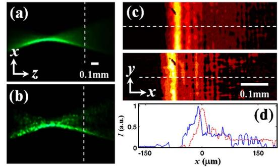
Fig. 5. (Color online) Experimental side-view photography of (a) linear and (b) nonlinear NAB. (c) Transverse output patterns taken at about  $z = 1$  mm as marked by dashed line in (a), (b), where top and bottom panels correspond to patterns from (a) and (b), respectively. (d) Linear (dashed) and nonlinear (solid) output intensity profiles taken along dashed line in (c).
