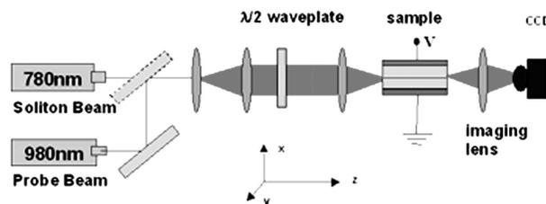
Fig. 1. Schematic drawing of the experimental setup.
