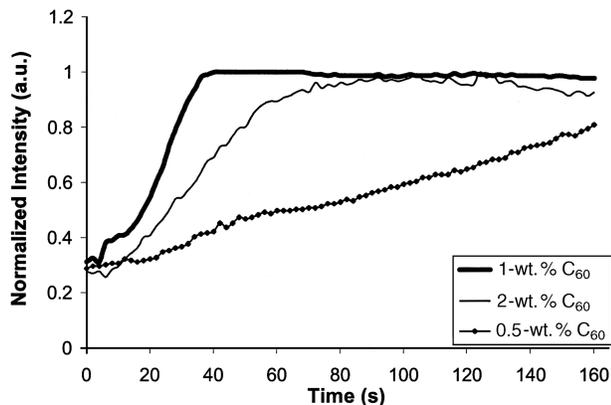
Fig. 4. Normalized peak intensity versus time for samples with various weight percent values of  $C_{60}$  at an applied field of  $13 \text{ V}/\mu\text{m}$ .
