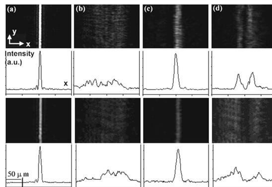
Fig. 2. Planar waveguides induced by 1D solitons. Shown are intensity patterns and beam profiles taken at (a) input, (b) linear output, (c) nonlinear output, and (d) output of (c) at turn-off of the field. Top, 780-nm soliton beam; bottom, 980-nm probe beam.
