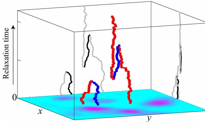
Fig. 5. Topological transformation of the off-site vortex on a square flexible lattice. Trajectories of vortices are shown vs. lattice depth (relaxation time  $t$  after blocking the lattice beam at  $t = 0$ ). The red lines (gray projections) correspond to vortex dislocation of charge  $+1$ , while the blue lines (black projections) correspond to charge  $-1$ .
