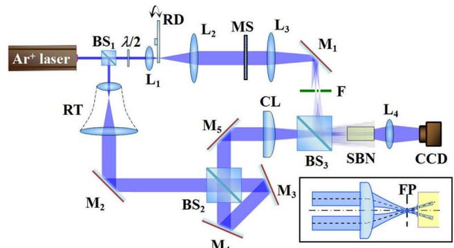
Fig. 3. (Color online) Experimental setup for observing coherent interactions between gap solitons: SBN, strontium barium niobate; BS, beam splitter;  $\lambda/2$ , half-wave plate; RT, reversed telescope; RD, rotating diffuser; L, lens; MS, amplitude mask; M, mirror; F, Fourier-plane filter; CL, cylindrical lens; and FP, focal plane.
