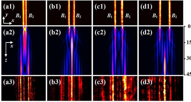
Fig. 4. (Color online) Experimental observation (top panels, input; bottom panels, output) and numerical simulation (middle panels) of in-phase gap solitons interacting in an optically induced photonic lattice. The initial beam separation in (a)–(d) is  $D = d, 2d, 3d,$  and  $4d$ , respectively.
